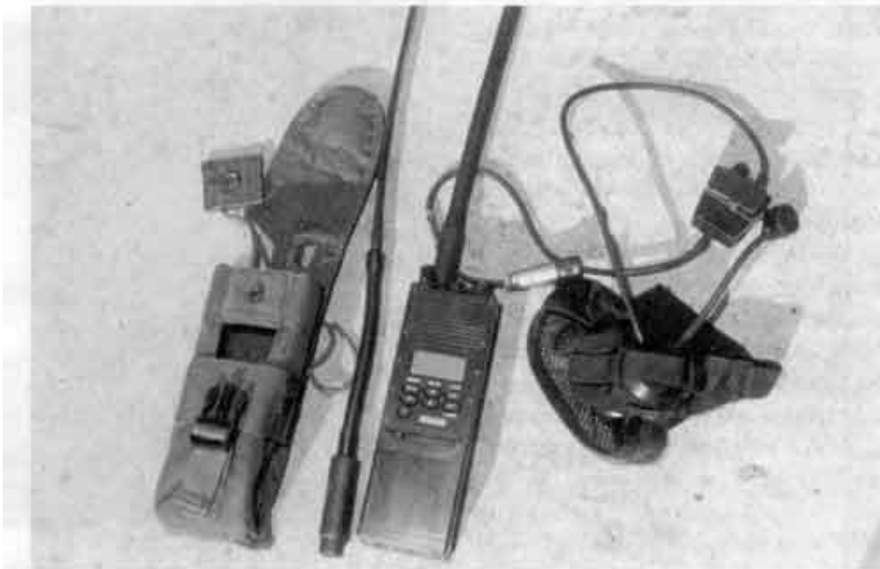
The MBITR Tactical Radio. It is UHF, VHF, embedded crypto and has a survival beacon. The Pouch is from Eagle Industries.
