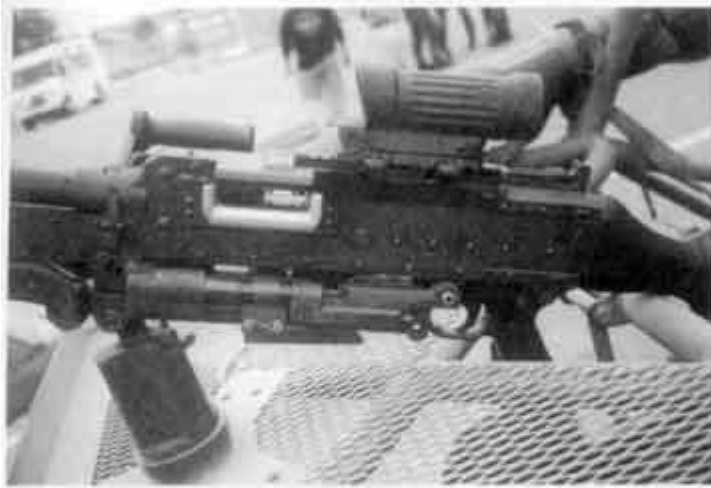
The M240G mounted on a FAV. The throw lever mount holds an Elcan.
