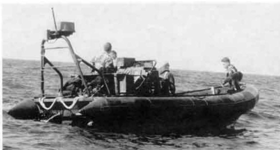
A RHIB providing plane guard for USS Duluth during the Osprey OpEval.
