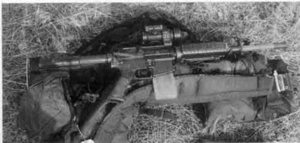
M4A1 Carbine with the SESAMS. This Simunitions™ kit permits force on force to be realistically accomplished. The barrel is blue, and the magazine is clear plastic and of a different configuration to prevent a mix up.
