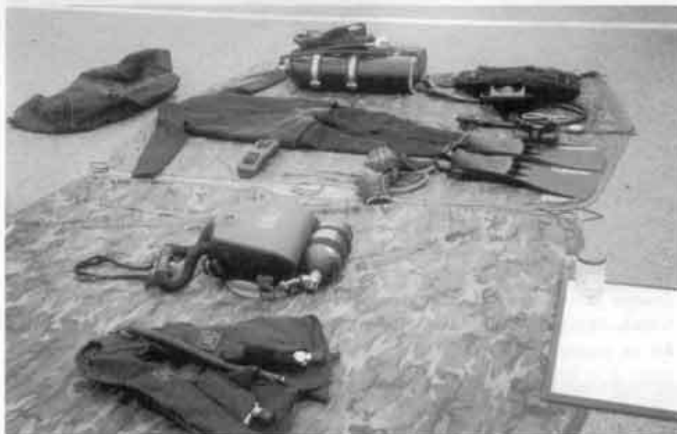
Divers gear laid out for display. The MK25 Mod2 Draegar is in the center. The Open Circuit equipment at the end of the display is for administrative support use only. The Draeger is used for all Combat Dive operations.
