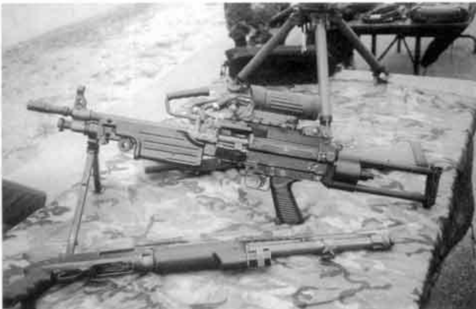
An M249 SAW (para). This gun has an Elcan optic, but does not have the RAS forend. In front of the SAW is a Remington 870 breaching shotgun.
