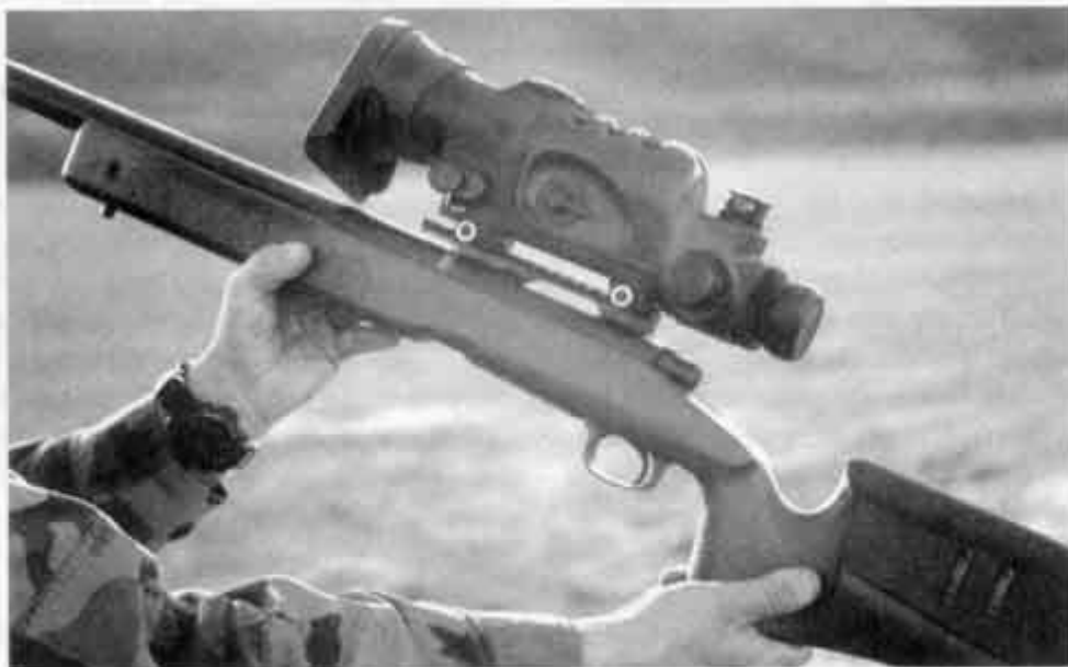
M40A3 with the AN/PVS-10. The mounting permits an eye relief similar to the Unertl telescope.
