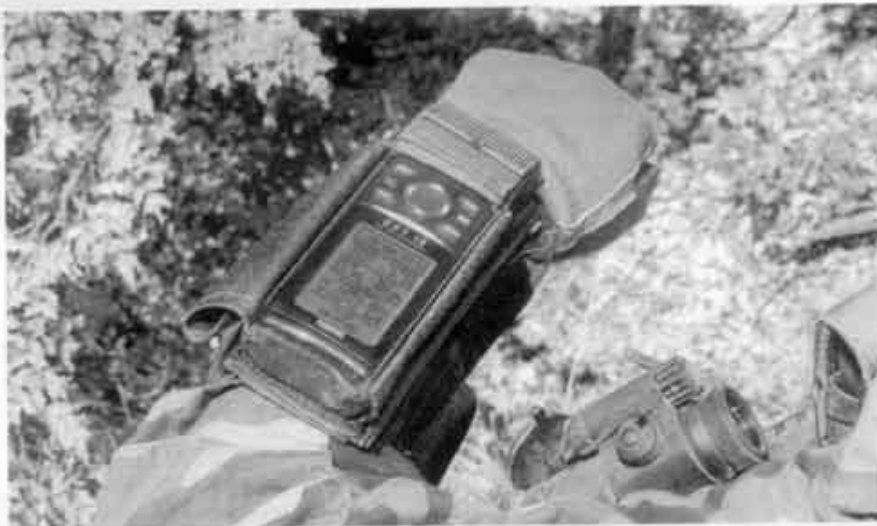
Each member of the Company has a Garmin model 12 GPS. This GPS is in an arm mount made in house by 3d Plt. Team Leader SSgt Matt.
