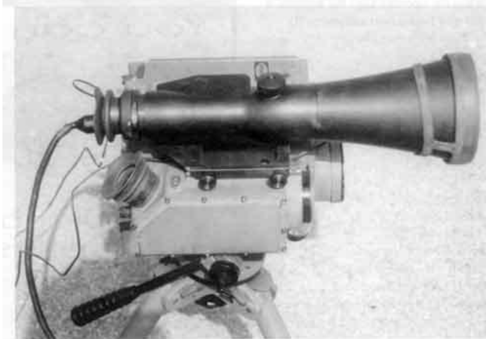
The AN/PEQ-1A SOFLAM, with an AN/PVS-13 Night Vision Sight on top. This is a lightweight, day/night man portable laser target designator and rangefinder.
