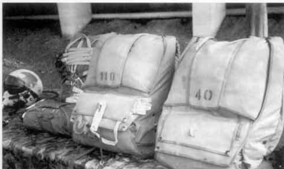
MC-5 Parachutes. The one on the right is for Military Freefall; the one on the left is rigged for static line. The smaller assemblies on the left are the MC1-1C Low Level Static Line Main and T-7 Reserve.
