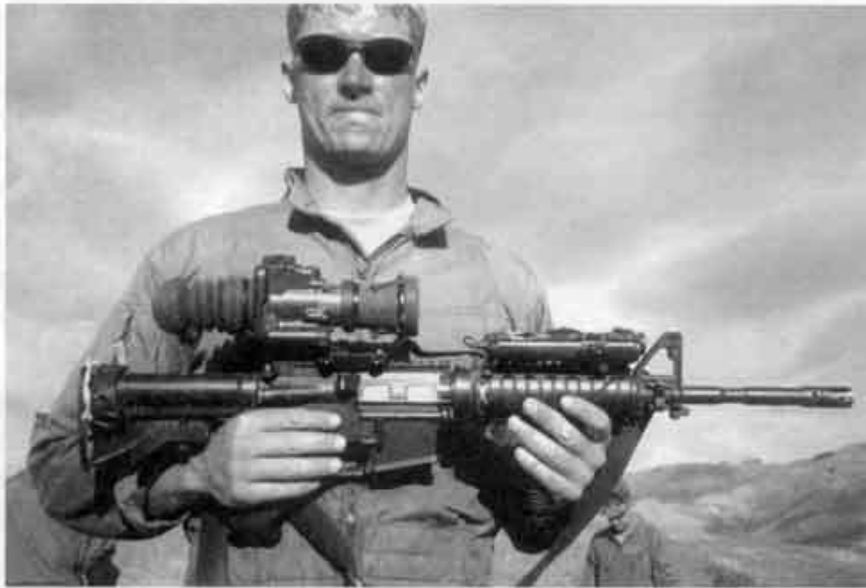
M4A1 Carbine with the AN/PVS-17 Mini Night Vision Sight mounted on the receiver, and the AN/PEQ-2 Infra-Red Target Pointer/Illuminator. Aiming Laser mounted on the RAS.
