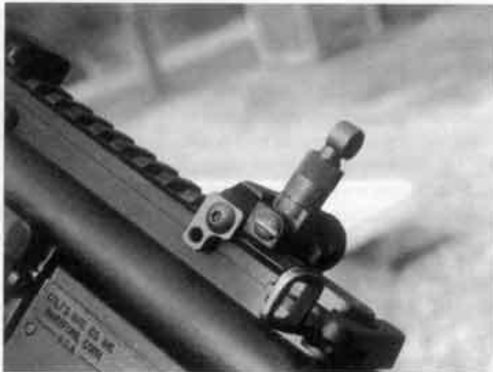
The Knight's Armament Corporation Back Up Iron sight (BIS). This is the 600 yard adjustable sight, P/N 98474). The Badger Tactical Latch is on the charging handle.
